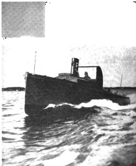
One of Four Torpedo Chasers Built by the Greenport Basin, Co. for Use on the Test Grounds of a Torpedo Factory. Length 37½ Ft., Beam 7½ Ft. Engine 35-H.P. Sterling. Speed 12½ Miles per Hour
